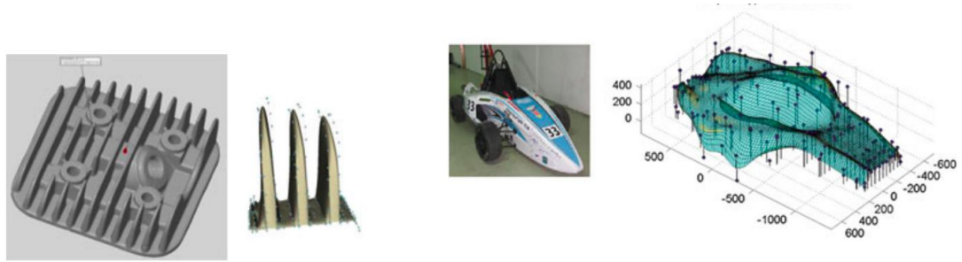
(a) 3D geometric parameterization of portion of small cylinder head.
